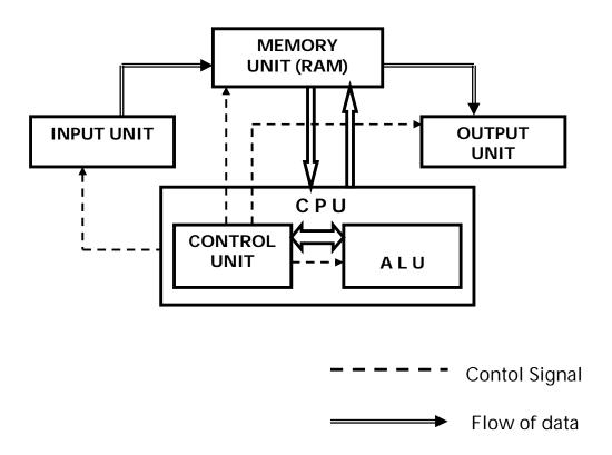
Usually the input given by the user will flow and store into Memory unit (RAM), then the given input will be checked by Control Unit then it transfers the input to the Arithmetic Logic Unit (ALU). The ALU processes such data according to the instructions given by the user and it again resends the output (result) to the Memory Unit (RAM). Then the output will be taken by the user the user through output devices such as Monitor and Printer.
